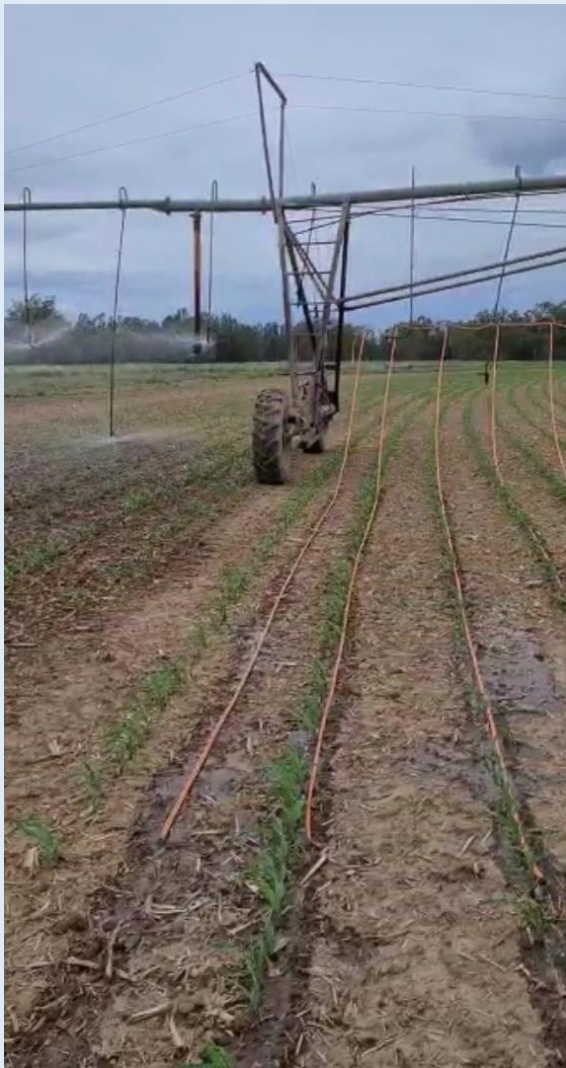
Figure 2 Mobile Drip Irrigation versus sprinkler emitters on a Centre Pivot Irrigator
